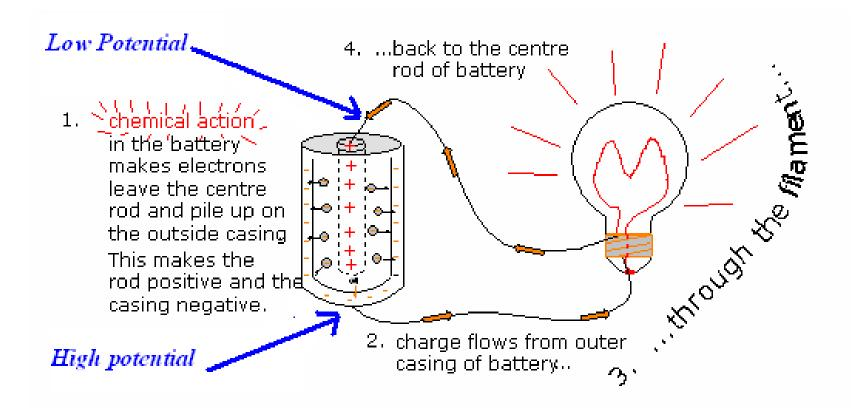
Electrons flow from regions of high Potential Energy to regions of low Potential Energy (something like the pile driver falling in the Potential Energy slide earlier) In the diagram electrons loose energy because of friction in the wires and the filament of the lamp.
