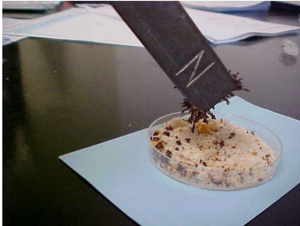
Removing iron filings from a mixture
