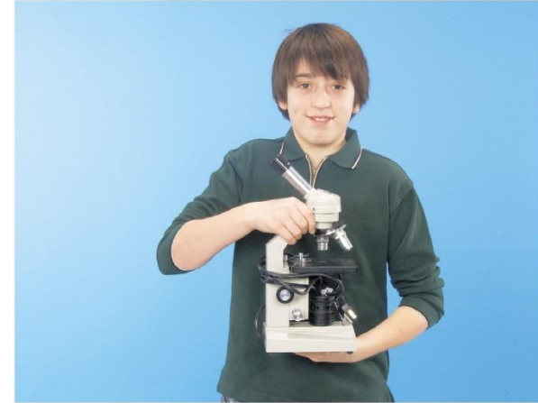
Figure 10.2 Always carry a microscope with one hand on the arm and one hand on the base.
