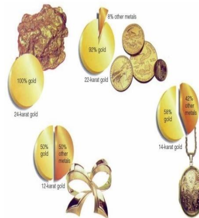
Figure 7.11 The pie graphs show the percentages of gold and other metals in different "gold" objects. Which of the objects shown here are pure substances? Which are homogeneous mixtures (solutions)?
