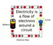
**Current (I)** refers to the flow of charges in a circuit. It is the amount of charge passing a point every second. It is measured in Amperes or Amps (A).
