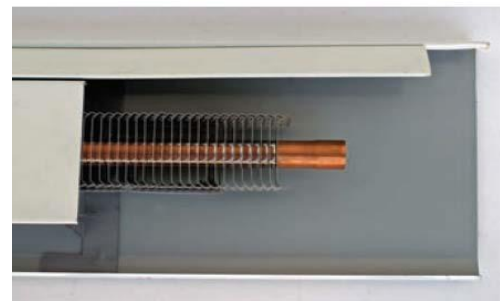
Figure 6.18 Baseboard heaters and radiators heat air by conduction with the air particles that come in contact with the metal surface. The hot air distributes the heat throughout the room by convection.
