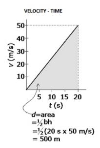
• The slope of a velocity-time graph is the acceleration
