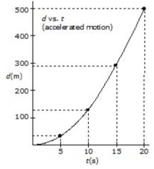
• To find the instantaneous velocities on the d-t graph, we draw **tangents**. Tangent is a straight line that touches a curve at only one point. Each tangent on a curve has a unique slope, which represents the velocity at that instant. In order for the object to be at that position, at that time, it must have an instantaneous velocity equal to the slope of the tangent at that point
