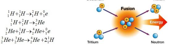
Because of the large binding energies involved in a nucleus, both fission and fusion involve energy changes of more than a million times larger than those energy changes associated with chemical reactions.
