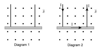
10. Two thin metal rods, A and B, are supported in a vertical wooden rack as shown in the diagram. The two rods are connected by a wire on one end and to a battery at the other end. It is observed that as the connection to the battery is made, one of the rods jumps upward. Identify which rod jumps upward and explain why. AUGUST 2008
