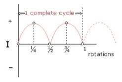
Real generator has many loops. Now look at a DC generator with two loops--one perpendicular to the other. Each loop has its own set of split rings. Notice just as the black loop loses contact with the brushes, the brown loop takes over. A plot of the current from a two-loop DC generator is shown.
