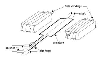
the main components of a generator are:
