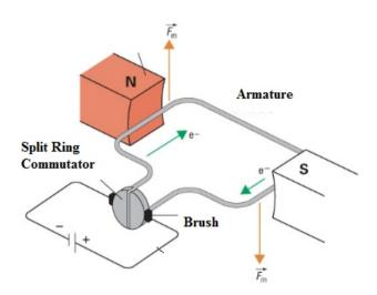
In the DC generator, the split half rings turn with the coil. The current is always going the same way in the external circuit. The needle of the galvanometer fluctuates from 0 to the + end as the loop goes from the vertical position to either one of the horizontal positions. The current in the external circuit never reverses, even though it does reverse in the generator loops. The current graph for a DC generator
