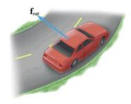
This acceleration is called **centripetal acceleration** and is always directed towards the center of a circle.
