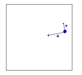
An object undergoing uniform circular motion is moving with constant speed; nonetheless, it is accelerating due to its change in direction. The direction of the acceleration is inwards
