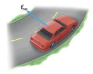
Any object moving in a circle (or along a circular path) experiences a centripetal force; that is there must be some physical force pushing or pulling the object towards the center of the circle.
