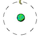
As the moon orbits the Earth, the force of gravity acting upon the moon provides the centripetal force required for circular motion.
