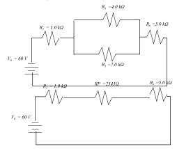
$$\begin{split} R_T &= 8545~\Omega;~I_0 = 7.0~x~10^{\text{-}3}~A,~Thus,~I_P = I_0,~so\\ V_{Branch} &= I_0~R_B = 17.82 V;~I_2 = V_B /~4000\\ I_3 &= V_B /~7000;~I_2 = 4.45~x~10^{\text{-}3}~A;~I_4 = 2.54~x~10^{\text{-}3} \end{split}$$
