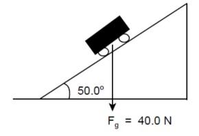
4. A box is held at rest on a frictionless incline as shown below. What is the tension, T, in the rope?
