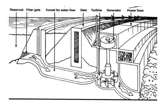
The water stored in the reservoir is used to make electricity. This hydroelectricity can provide power to homes and businesses. Just like a waterfall, water from the lake gushes through narrow openings inside the dam. The water hits the blades of **turbines**, or engines, and causes them to spin. These engines power the generators that make electricity
