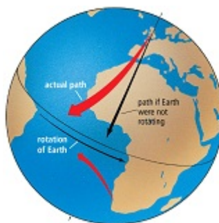
Figure 11.13 The Coriolis effect, caused by Earth's rotation, results in the path of air being directed clockwise in the northern hemisphere and counter clockwise in the southern hemisphere.
